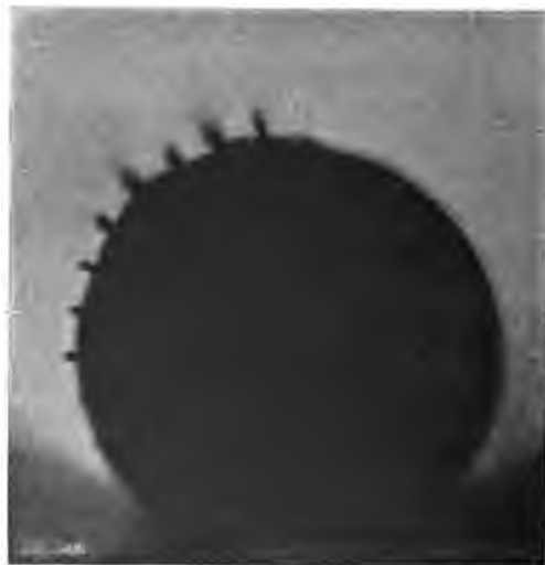
FIG. 37.—In this case a layer of paraffin 8 mm. thick is placed over the outer holes.
